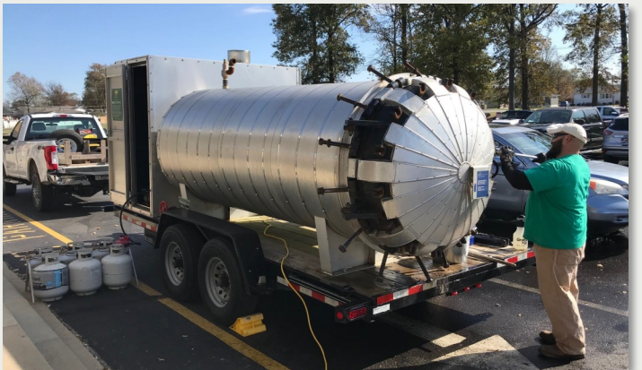
J.J. locking down the door of the KSU Autoclave. Each locking bolt is torqued properly.
